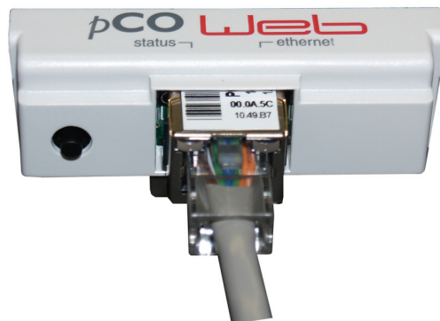
Figure 4-5. BACnet IP, BACnet Ethernet, HTTP, SNMP, and Modbus IP BMS interface port.
